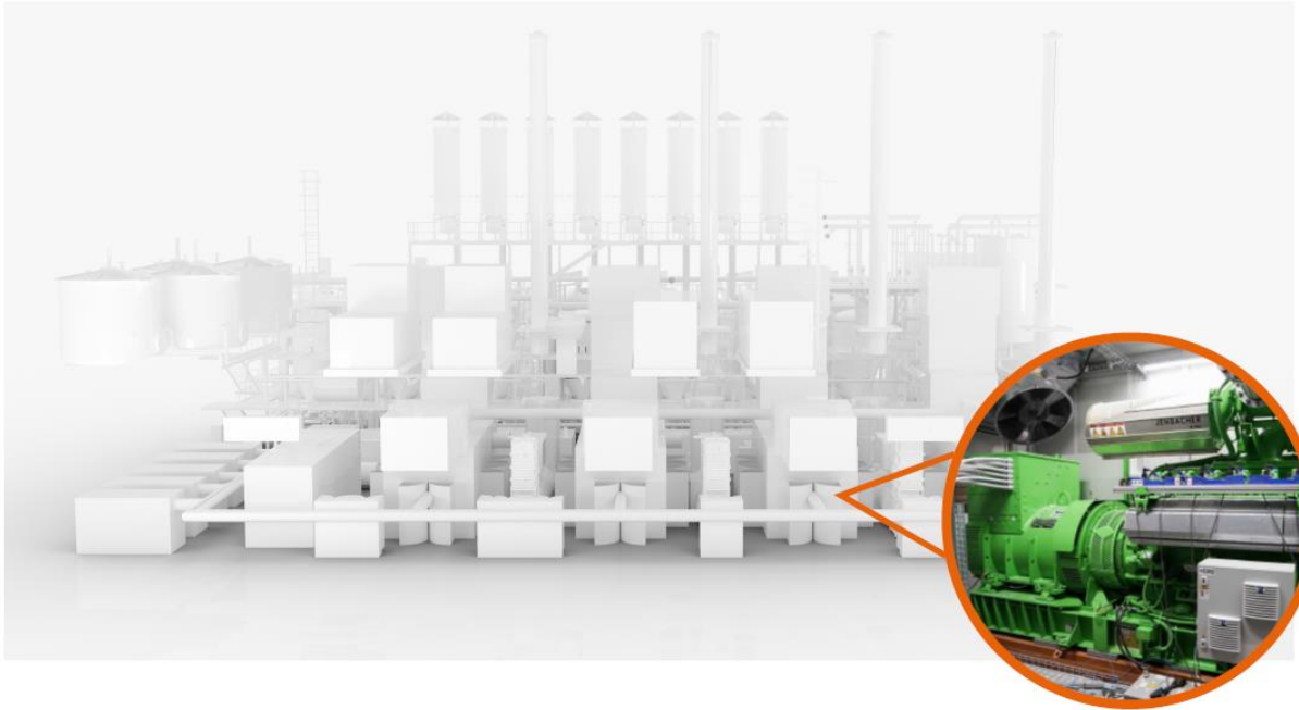
Four special gas engines convert the wood gas produced from biochar into electricity and renewable heat. Source: Bioenergie Frauenfeld AG, 2022.
